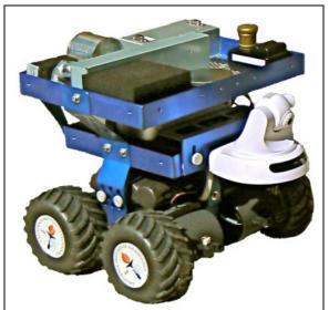
The CYCLOPS mobile robotic platform is designed to be used as a surrogate for blind persons in the testing of visual prostheses.
